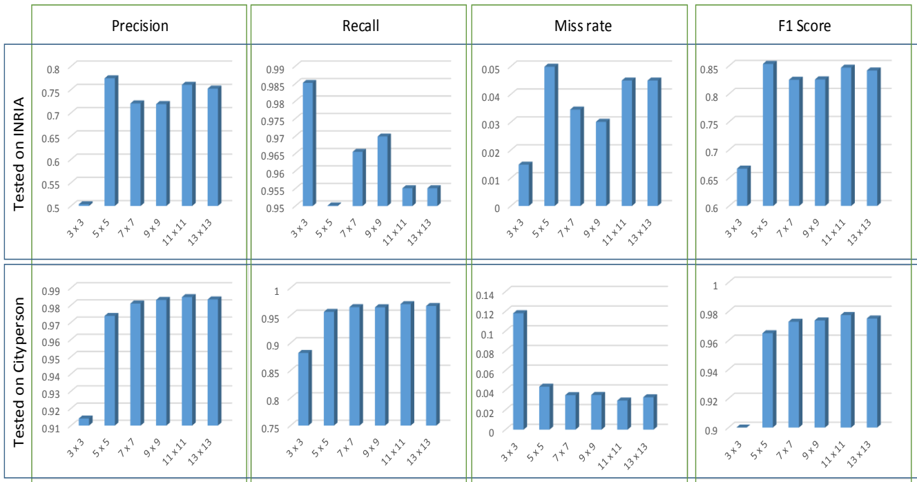
Fig. 4. Classification Performance against Filter Size. The CNN is trained with CityPersons
