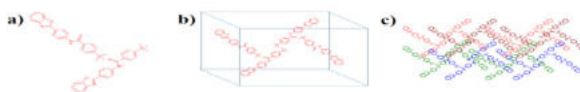
Fig. 9: a) Cross Aggregate of OTB, b) Four Molecules in A Single Unit Cell, c) 3-D Propagation of the Packing in Single Crystal (W. Huang et al. 2012)
