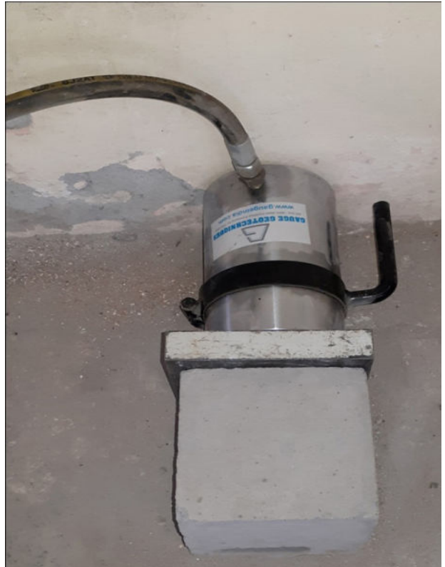
Fig. 13: Specimen for Horizontal Shear Test Bonded on the Existing Concrete Floor, with Hydraulic Jack for Load Application
