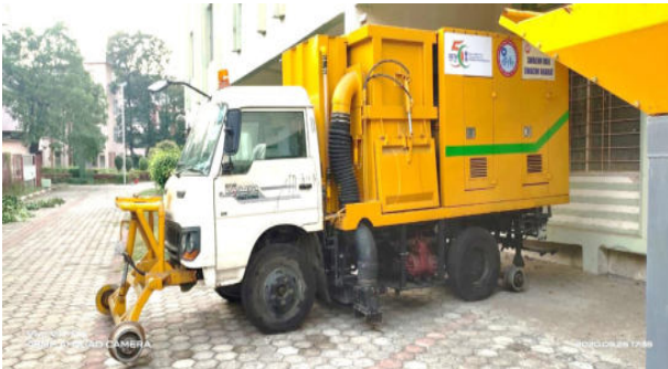
Fig. 1: Designed and Developed Rail Track Scavenging Vehicle
