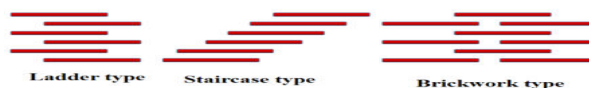
Fig. 1: Various Parallel Packing Pattern of the Organic Molecules in Crystals (A. Vannikov et al. 2012)
