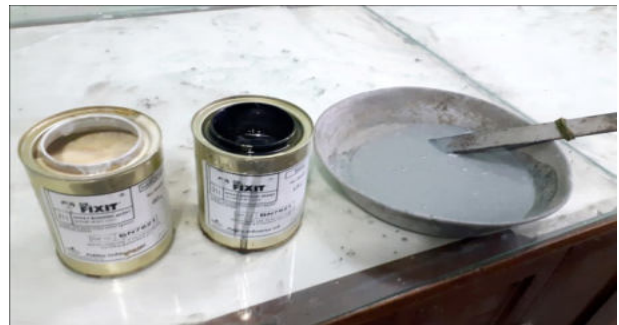
Fig. 3: Epoxy Base and Hardener Used (in Containers) and 1:1 Epoxy Paste (in Pan)
