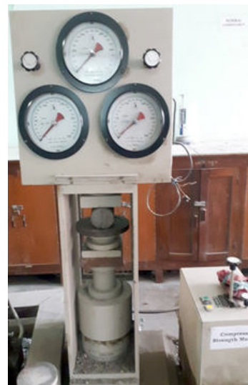
Fig. 5: Specimen for Split Tensile Test Placed in Apparatus
