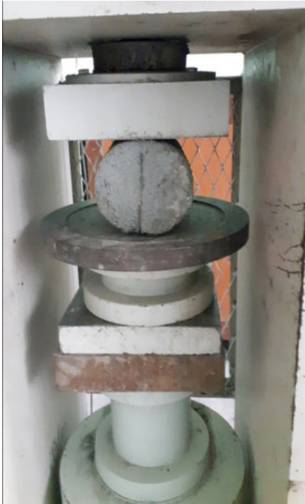
Fig. 6: Specimen for Split Tensile Test Placed
