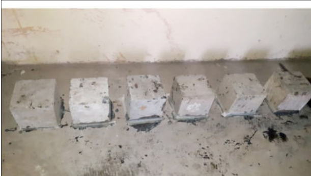
Fig. 15: Six Specimens for Horizontal Shear Test Bonded over an Existing Rough Concrete Floor, Bonded using Epoxy
