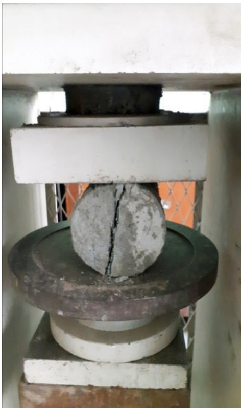
Fig. 7: Split Specimen Along a Bonded Plane at Ultimate Load in the Split Tensile Test
