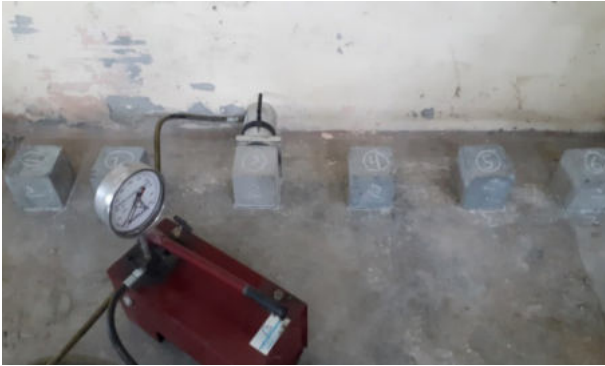
Fig. 14: Six Specimens for Horizontal Shear Test Bonded over an Existing Rough Concrete Floor, Bonded using Cement Slurry with Hydraulic Jack Assembly also Seen, Used for the application of Horizontal Load
