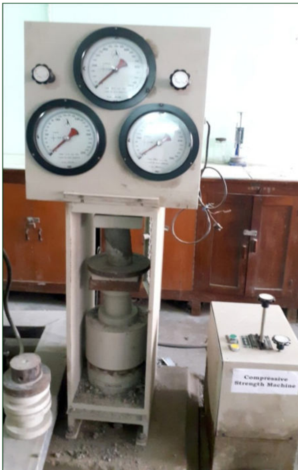
Fig 10: Specimen for Slant Shear Test Placed in Apparatus
