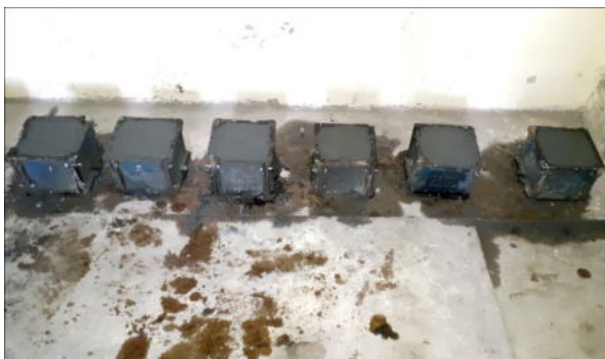
Fig. 16: Six Concrete Cubes case in-situ over Concrete Floor to Perform Horizontal Shear Test
