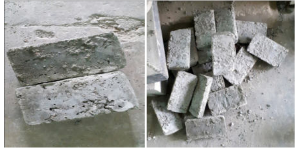
Fig. 8: Split Specimens Along Bonding Plane, Cement Slurry as the Bonding Agent
