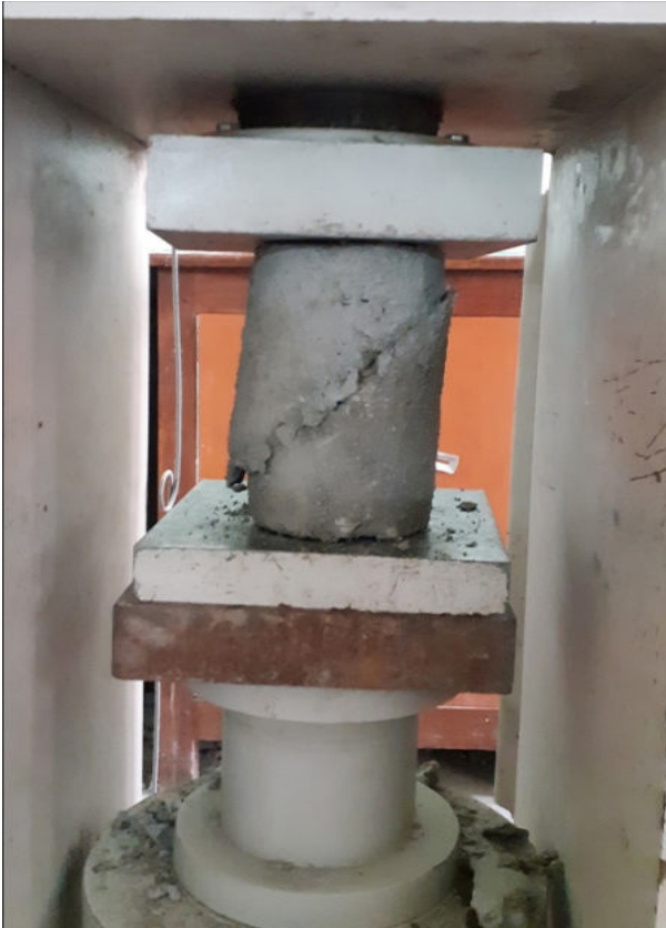
Fig. 12: Split Specimen along a Bonded Plane at Ultimate Load in Slant Shear Test
