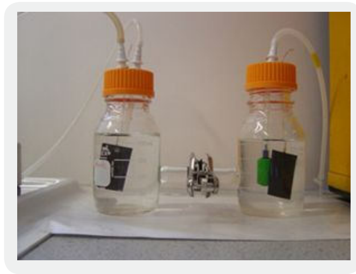
Figure 2: A simple two-chamber system microbial fuel cell [29]
