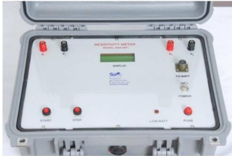
Fig. 2.1. Electrical Resistivity Meter (Model: SSR MP1) used for the present study.
